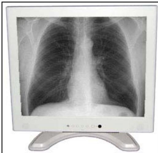
19 inch LCD with a 4:3 aspect ratio. This unit is water sealed with an anti-glare glass front. Capable of 16.7 million colors and a resolution of 1280 x 1024. The 19 inch monitor has a viewing angle of 170 degrees and a response time of 15/10 ms. This unit is cart or wall mountable and has video inputs for VGA, Composite or S-Video. The monitor is compatible with NTSC, PAL or SECAM.
